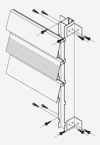
Installed vertically or horizontally, Fácil Façades' louvers are available in many profiles and finishes.
